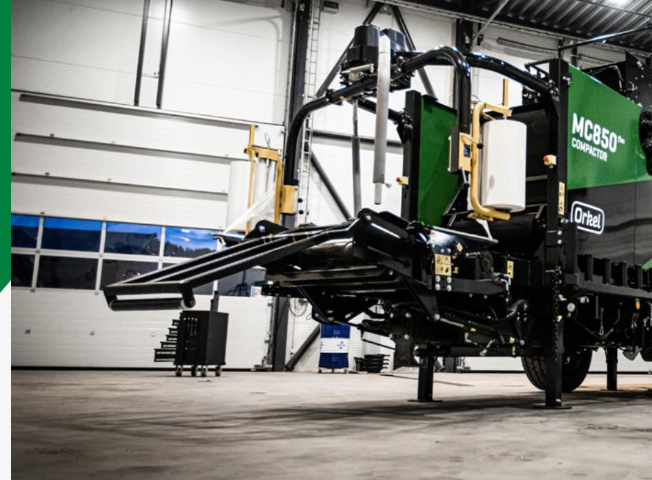
The weight of a flex bale starts at approximately 100 kg, and may range up to 450 kg, according to customer preference. Compared to the initial MC850 model, the MC850 flex model is equipped with a kit and specialized bale settings, limiting the bale diameter to 50 cm. Furthermore, the compactor's wrapper unit is re-sized to fit a 200 - 300 mm wide wrapping film. Combined, the additional characteristics of the MC850 flex model creates an easy-to-handle compactor unit.
